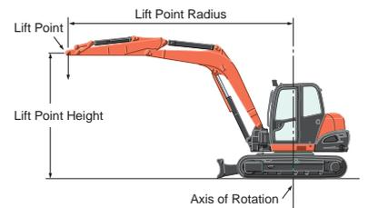
\* Working ranges are with Kubota standard bucket, without quick coupler.
